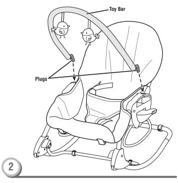
• Fit the plugs on each end of the toy bar into the sockets in each side rail.
